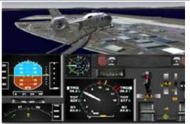
IRIS HAS A COMPREHENSIVE SUITE OF SOFTWARE TO PLAYBACK AND ANALYZE THE RECORDED DATA. THE FLIGHT ANALYSIS SAFETY TREND AND REPORTING SYSTEM (FASTARS) SOFTWARE SUPPLIES VOICE AND VIDEO PLAYBACK TOOLS ALONG WITH MODULES TO CREATE FLIGHT AND MAINTENANCE OPERATIONAL QUALITY ASSURANCE (FOQA/MOQA) EVENTS, ANIMATIONS AND SECURE DOWNLOAD TOOLS CUSTOMIZABLE BY THE CUSTOMER.
